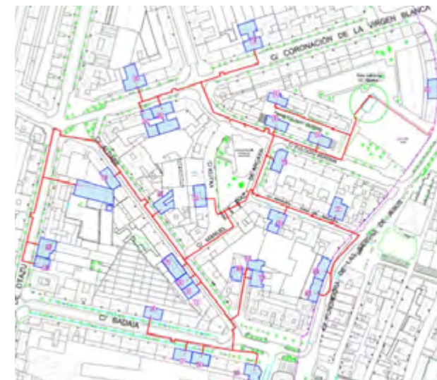
Biomass district heating system in Vitoria-Gasteiz, Spain ©SmartEnCity
