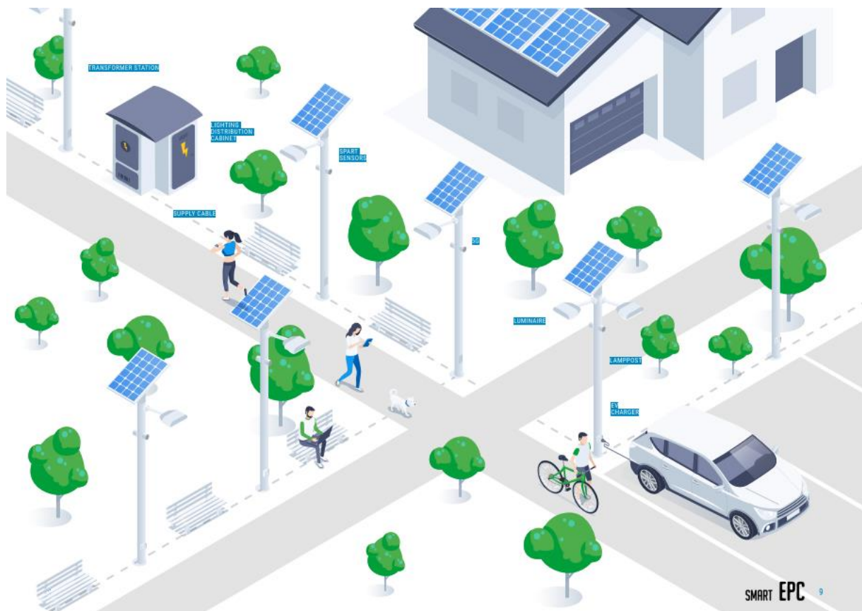
Figure 2 Visualisation of public lighting system basic elements
